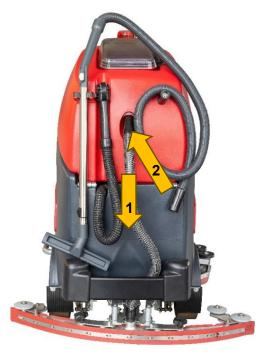
Remove the suction hose from the top of the machine's suction nozzle (1) and fit the suction hose from the water suction set (2).
