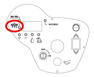
A long press of the suction function button (> 3 seconds) switches the suction function on even when the machine is stationary; the driver's seat does not have to be occupied. When the work is done, switch the suction function off again by briefly pressing the button.
