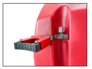
Then remove the existing dirty water hose holder (left image) and replace it with the new hose holder. Use the existing screw for this. (Image on the right)
